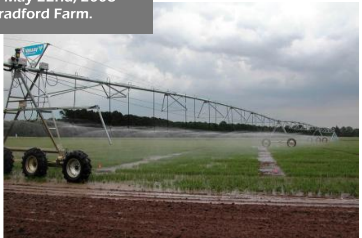
Center pivot irrigation on one of Gene Steven's rice experiments near Portageville, MO. Gene is investigating the potential for reducing water usage for the rice crop using sprinkler irrigation compared with the flood system.
